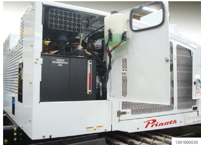
Figure 138 Lateral right side access panel (rear) - engine oil dipstick, oil tank filler neck and sight glass, engine air filter, windshield washer fluid tank and track tension release buttons (rubber track vehicle)
