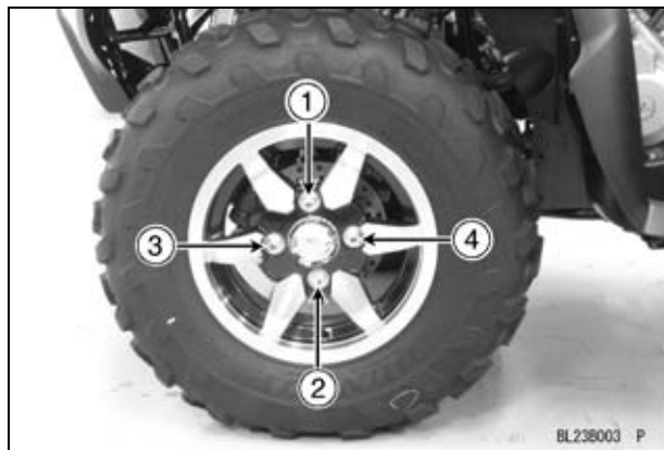
Nut-Tightening Pattern
