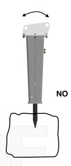
If you insist on the same spot for a long time, the drill can swell up, the tool can seize and the oil can become overheated.
