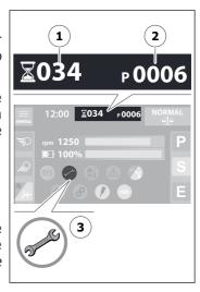
After completing the maintenance operations, the *Service Centre* will reset the maintenance interval hour meter, via the specific SERVICE page, so that the indicator light (3) goes out.
