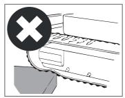
Prevent foreign bodies from getting stuck between the track and the frame or the components of the undercarriage; if this happens, the entire undercarriage may be damaged and the track may be deformed and/ or cut.
