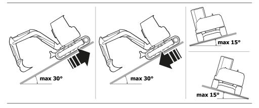
When travelling on a slope with an angle lower than 15°, always reduce the machine speed and maintain a slow, steady motion. Apply braking by smoothly returning both travel control levers to the NEUTRAL position (N).
