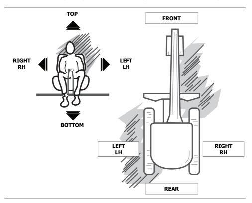
For ease of use and maintenance, the following are the names of some of the machine parts, which will be referred to in the descriptions provided in the manual.
