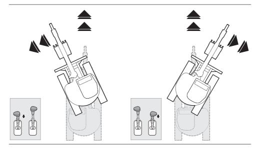
With the machine travelling straight **FORWARD,** both control levers must be pushed forward by equal amounts.
