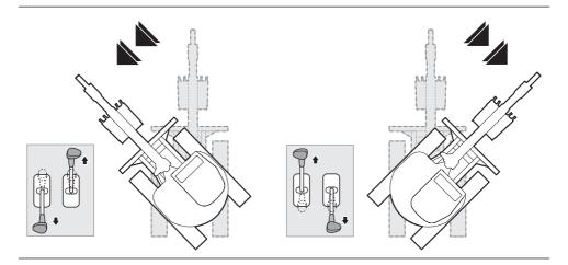
To pivot the machine to the **LEFT** on its axis, push the right control lever forward while pulling the left lever to the rear.
