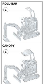
If at least one of the above problems is found, contact the *Service Centre* to have the structure checked and restored. The protective structure protects the operator from the risk of crushing in the event that the machine tips over or rolls over.
