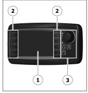
The operator can interact with the display either with the **no. 8 function keys**, located on either side of the screen, or with the navigation **hand grip** (4) and the buttons **Home** (5) and **Reset** (6) located to the right of the display.
