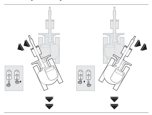
With the machine moving straight in **REVERSE**, both control levers must be pulled back by equal amounts.
