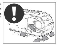
Protruding bodies should be avoided, if possible. If this manoeuvre is not possible, proceed with care at low speed and moving in a straight direction without steering when the track is over the obstacle.
