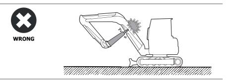
Do not use the demolition hammer with the second boom in a vertical position; excessive vibration on the second boom may cause oil leaks.
