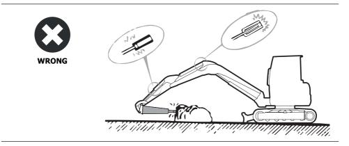
Do not operate with the demolition hammer in a sideways position; the machine will become unstable and the undercarriage components will be subjected to increased wear.
