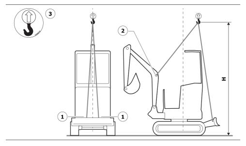
**H** Minimum ground height of the anchoring point
