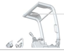
Protective structure ID plate (roll-bar)
