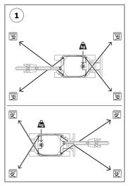
To avoid damage to the anchoring elements and/or to the anchor points of the machine, use guards for sharp edges.
