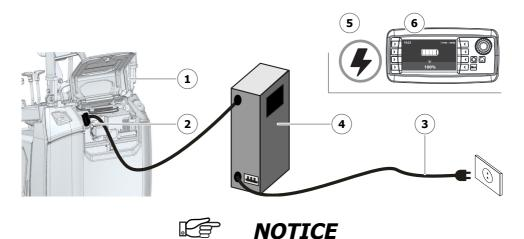
Keep the rear cover open during charging to allow the heat to be disposed of.
