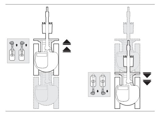
To begin **FORWARD** travel, move both control levers forward equally. As additional pressure is applied on the control levers, the machine speed will increase. To STOP the forward travel, return slowly both controls to their NEUTRAL (N) position.
