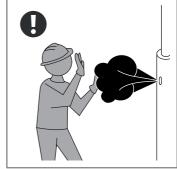
Pressurised fluid leaks may be invisible. **DO NOT** use hands to check for leaks. Use a piece of cardboard or paper to this purpose.
