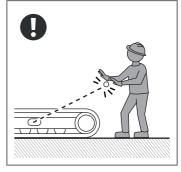
The cylinder that adjusts the track tension is filled with grease; therefore the grease itself may be under high pressure. Under this circumstance, if the plug is loosened carelessly, both the plug and the lubricant may get pushed out causing a dangerous situation.
