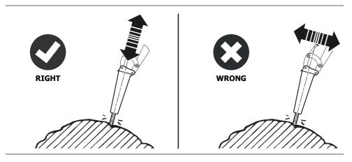
Do not operate with the demolition hammer for more than one minute in the same spot, since the tip and/or hydraulic mechanism may get excessively worn; if the object does not break within a minute, place the tip on another spot.
