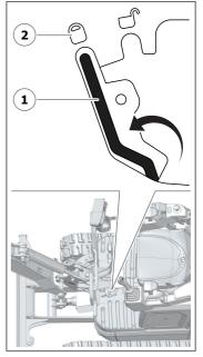
Always lock the slewing when transporting the machine and at the end of each day of work.
