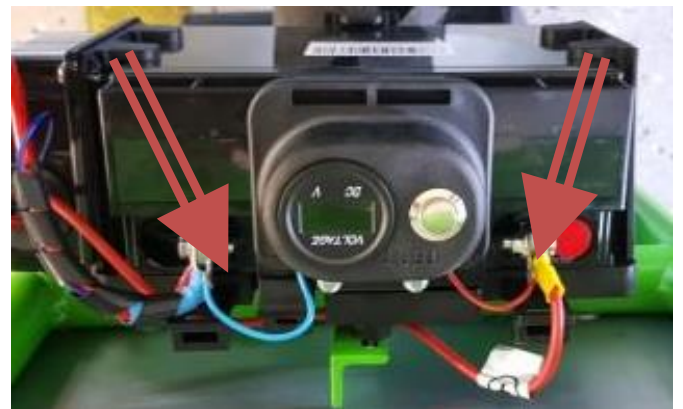
pict. 8. – marking the place where the the battery is unscrewed from the wires
