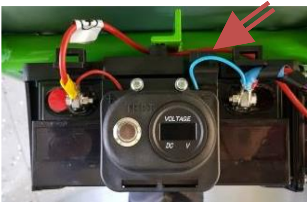
pict. 7. – disconnecting the battery from the holder
