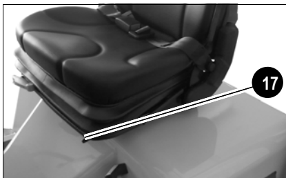
Fig. 62: Horizontal seat adjustment
