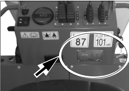
Fig. 1: Position of the type label
