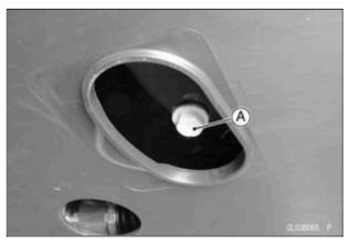
A. Engine Oil Drain Bolt and Gasket
