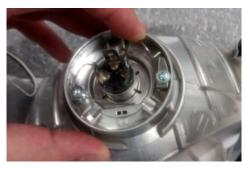
5. Install the new bulb into the housing.
